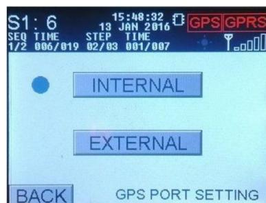
Figure 26: GPS Type Selection Screen
