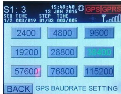
Figure 27: Baud Rate Selection Screen
